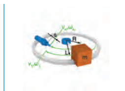
R6. Horizontally pivoting mass with form-fit drive torque
